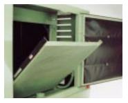
Swing-Down Cooler Permits easy cleaning of both compressor cooler and the engine radiator.
