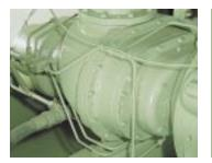
Rotary Screw Compressor Single-stage, fluid flooded, cast iron housing is dimensionally stable, thick walled and machined to close tolerances.
