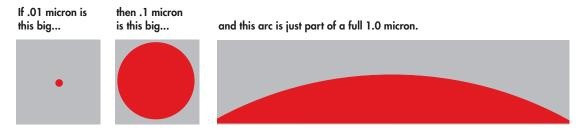
When you realize it takes 10 million particles 1.0 micron in diameter to cover this 1/8 inch dot
