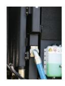
**DIFFERENTIAL PRESSURE SHUTDOWN SYSTEM FOR FILTERS**—This system senses differential pressures when filters require maintenance. If there is no response, the system automatically shuts down the machine, to ensure that no contaminant or oil is allowed to go beyond the filter. (Option on 300HH, 375, 375H, 375HH, 425 and 425H)
