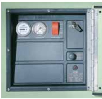
Curbside Instrument Panel With (SSAM) Shutdown System & Annunciation Module.
